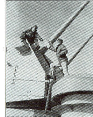
Checking the 5-inch twin gun mount.
