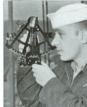
Old but reliable technology. The sextant is used to check the accuracy of the ship’s high tech gyrocompass.
